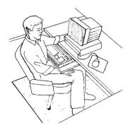
At work, you can manage static by using wrist-grounding straps, anti-static work surfaces and leather shoes. If necessary, you can place an anti-static shield over your computer monitor screen and anti-static mats under the chair, keyboard and mouse.
