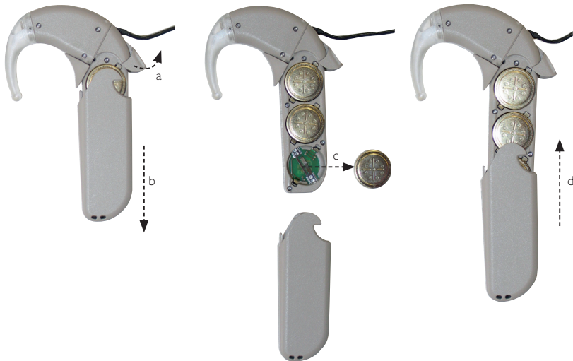
Fig. 16 Changing the batteries of your speech processor
