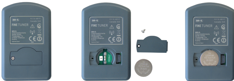
Fig. 17 Changing the battery of your FineTuner
