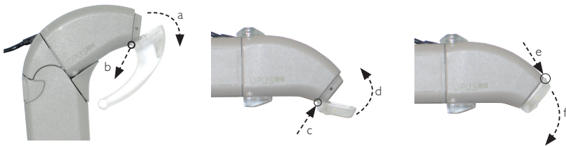
Fig. 14 How to remove the earhook or microphone cover
