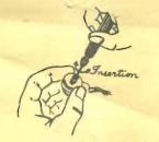
Screw the sound-tip clockwise, to be inserted. Screw it counter-clockwise to be released.
