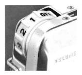
The new ROYAL CRUSADER features a smoothly rotating volume control permitting finger-tip adjustment of sound amplification for best hearing under varying acoustic conditions. The on/off switch is combined with the volume control. When instrument is not in use, always rotate wheel to "off" position to avoid exhausting batteries.
