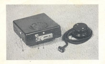
THE PYLON MODEL P hearing aid consists of a single unit housing microphone, miniature valve amplifier, low and high tension batteries. This unit can be worn in pocket, handbag, or hung round the neck by means of carrier which is clipped on study S on sides of instrument.
